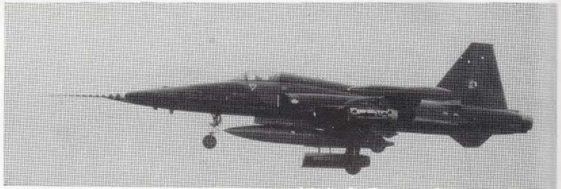
TWO F-5s. ABOVE: RNoAF F-5A 165 visiting Soesterberg. RIGHT: Klu Testgroep NF-5A K-3001. The two pods under the wings are used to study the behaviours of rocket-dispenser pods after dropping. (both B.Berkemeijer)
